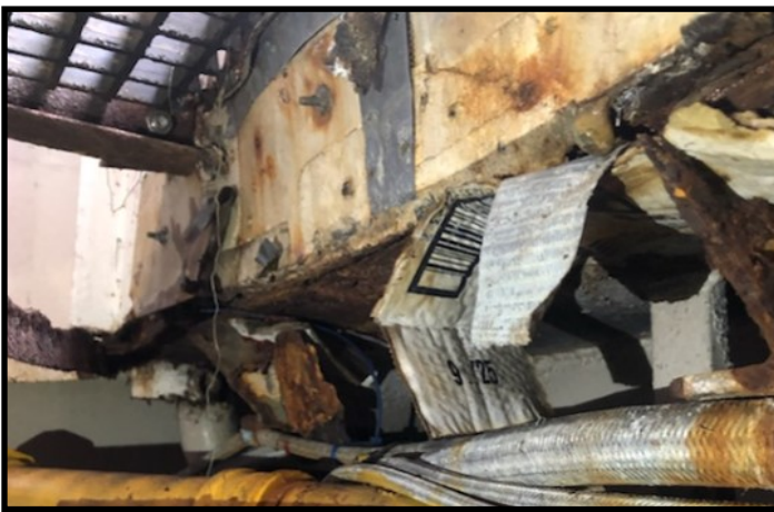
MSU Lake Charles ITV Detention (Cardboard & Duct Tape Covering Wastage/Rot of Main Deck)
